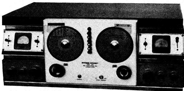
fig. 1. The tuner section only of a Hallicrafters DD-1 receiver. There was also a power supply chassis and an audio amplifier chassis. Dual S-meters sat on top of the receiver, all of which added impressiveness to the system.
