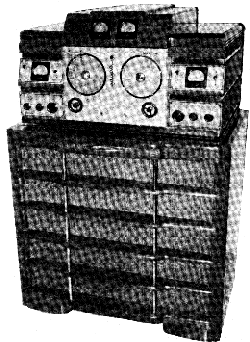
fig. 8. The late production or "jazzed-up" version of the DD-1 showing the special hi-fi loud speaker made by Jensen especially for this receiver. Note that the bandspread dial is blank. (Photo courtesy Charles Dachis, WD4EOG.)
