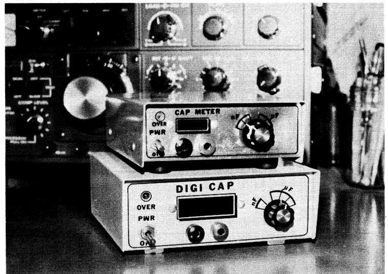
Two different meters showing suggested range switch labeling for right-hand decimal displays per the text (on top) and left-hand decimal displays. The unit with the small display (top) was used to develop the circuit. The bottom unit was built by WA4RVN to verify the circuit reproducibility and performance consistency.
